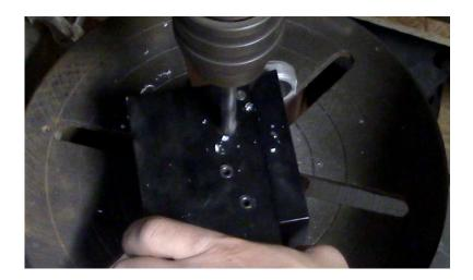
B. Use 5/32 drill bit to drill through both remaining holes through the entire lower on hardened drill bushing side.
