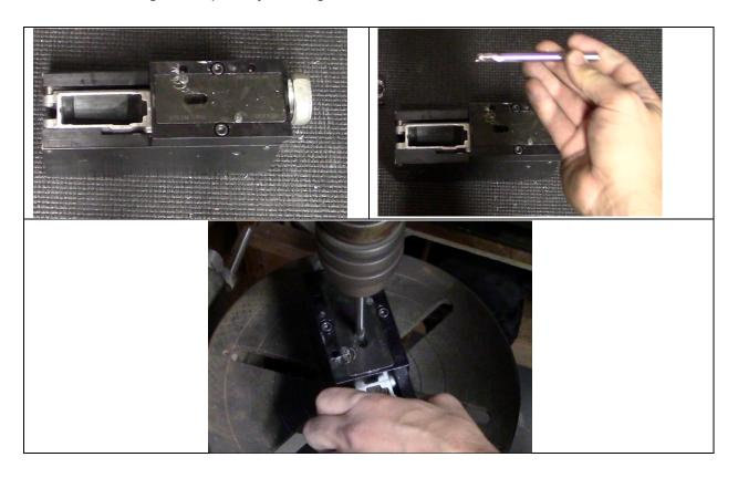
A. Use 3/8 bit to drill through the hardened drill busing side of the jig kit and go through both walls.
