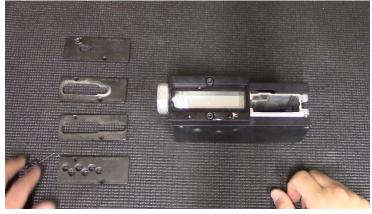
Set 1st plate (honeycomb style plate) into nest plate. Tighten down with the allen wrench and set screws that were provided.
